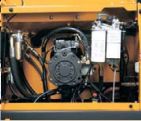
• Easy access to hydraulic pumps and filters.
