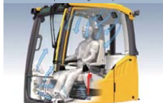
• Industry's highest heating/cooling capacity with 14 vents.
